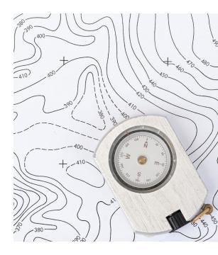
The distinctive characteristic of a topographic map is the use of elevation contour lines to show the shape of the Earth's surface.
